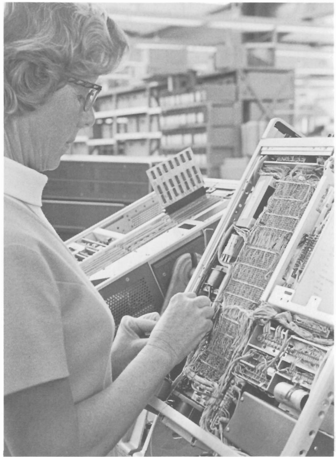
Nearing end of production line, maze of wiring is organized by Jean Gilles. Counter's back plane features more than 2,000 interconnections made by automatic machine.
