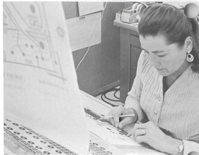
Versatile computational abilities of new counter are based in large part on extensive use of printed circuits and IC's. Here Gladys Kinney works on artwork for new PC board.
