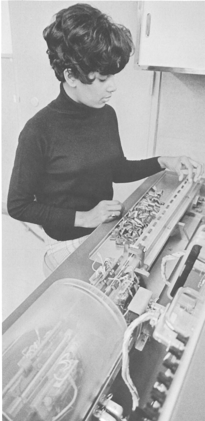
Of the 458 integrated circuits used in new counter, 86 have been designed and produced by HP. Here, packages of the miniature circuits receive final test on HP-designed test system operated by Evelyn Homel. Test puts ICs through hot, cold and room-temperature cycle.
